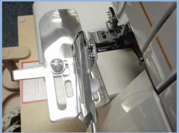
This is a new, high-quality Industrial-Grade Collarete Coverstitch Binder mounted on the BabyLock Evolve using our "L" Bracket. Note that the Binder is "angled" slightly toward the Presser Foot Area. The greater the angle, the closer to the Presser Foot the folded Binding Material will exit the Binder. Lastly, this Binder may be used with one or two of the white mounting screws, depending upon the angle used.
